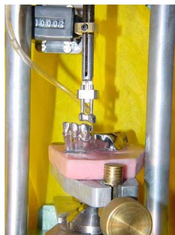
FIGURE 2. Insertion/removal cycling apparatus.
