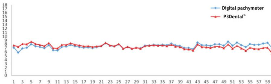
Figure 10. Distribution of measurements of the superior region of the sections.
